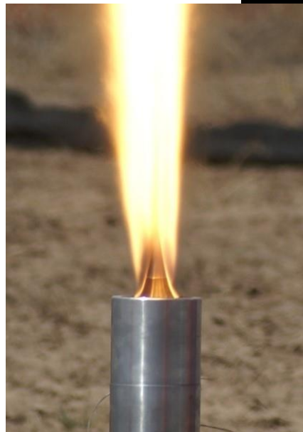
Independent research: a toroidal aerospike nozzle integrated with an N_2O /HTPB hybrid motor
