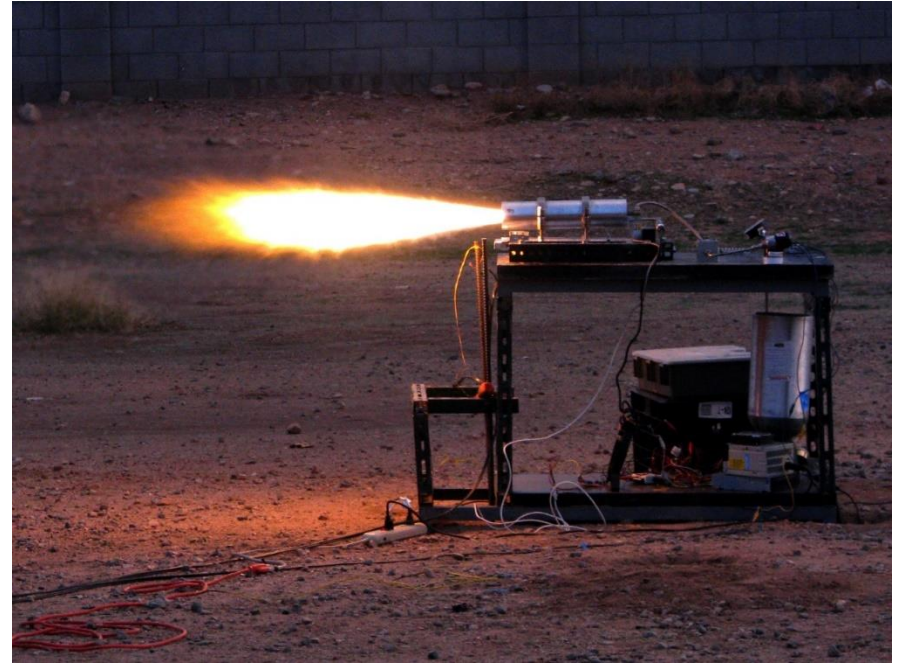
Test fire of hybrid rocket engine developed by Sun Devil Rocketry
